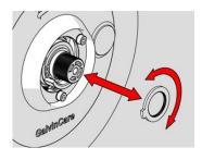
Remove the lower brass ring (temperature setting ring) and rotate the brass ring clockwise to increase temperature or anti-clockwise to decrease. Refit to spline in new position.
