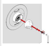
Unscrew the tamper proof screw from handle. Pull out handle assembly from the body
