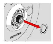
Remove the upper brass ring. Make sure the control rod doesn't rotate during the next steps.
